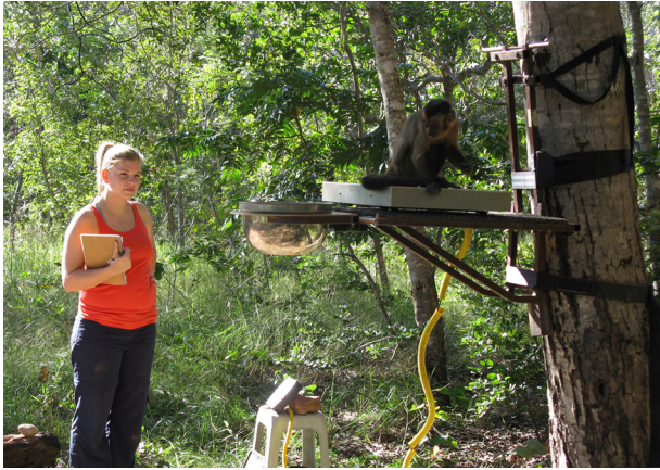
Fig. 1. Arrangement to obtain body mass of wild monkeys. A digital scale is mounted on the trunk of a tree in an area the monkeys visit regularly, and a bowl of water is placed at one end of the scale, so that a monkey visiting the water bowl passes over the scale platform. A digital display is placed a few meters away. A visual indicator appeared on the digital display when a stable mass was attained. We recorded an animal's mass only when it had four limbs on the scale platform and when the tail was not touching a surface other than the scale platform or was unsupported, and the monkey remained stationary long enough to register a stable mass value. Photo by S. T. Johnson.
